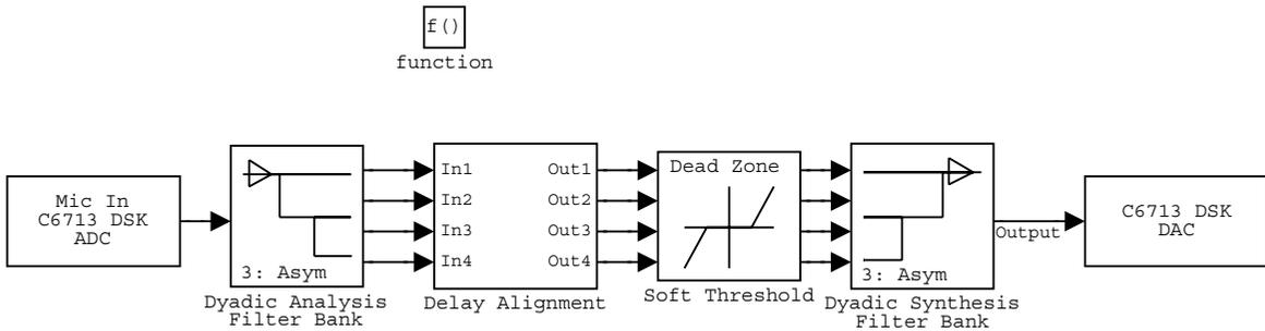
**Compatibility Consideration.** The V3.0 changes in the real-time scheduler can break some existing multirate models that contain codec blocks such as the ADC and DAC. The models affected contain at least one sample rate that is faster than the codec block rate. You do not run into this problem if all rates in the model are lower than the codec rate.
